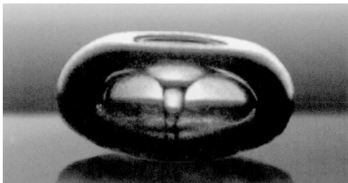
Multiple enlarged cavitation bubble at a frequency of 25 kHz during the implosion
